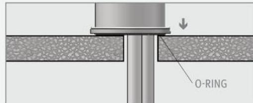
2 Slide the gasket, disk and hexagonal nut over the flexible hose and secure the faucet into place.
